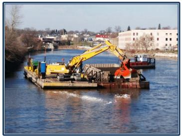
Figure 2 - Prototype environmental bucket designed for excavator use
